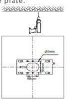
3. Place the plastic wall anchors in the holes. Affix the plate to the ceiling with screws and/or washers.
